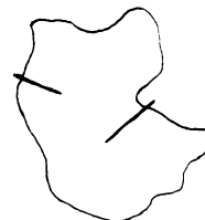
Fiber protrusion <0.5 micrometer
