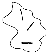
No fiber protrusion
