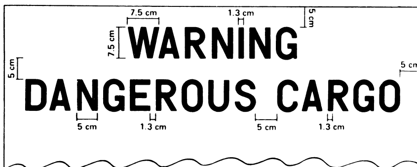
Figure 1 - Minimum Dimensions for Warning Sign
